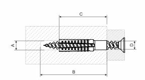
product description: For pre-assembled mounting in concrete, porous concrete, vertically perforated bricks, natural stone with a dense structure, solid brickwork blocks, solid sand- lime bricks.
