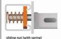
sliding nut (with spring) detail of bracket aachment to the profile with bolt S 10X20 and sliding nut with spring PMP 41 M 10
